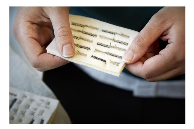
The dark yarn is the cellulose yarn and the lighter one is a commercially available silver-plated yarn, both of which are electrically conductive. The
