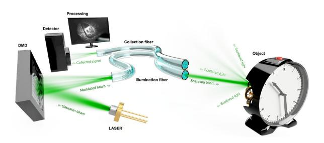
A sequence of holograms displayed by a digital micromirror device spatially shapes the wavefronts coupled into a multimode optical fiber in such a way that a far-field focus scans the distal field of view. Credit: Tomas Cizmar
