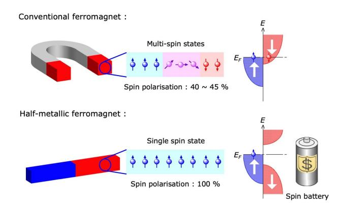
Spin 'batteries' use electron spins, instead of their charge, to power spintronic devices. Credit: ResearchSEA
