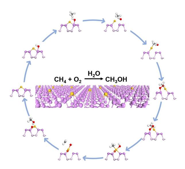
Schematic diagram of the reaction pathway for methane oxidation over Au1/BP nanosheets. Credit: LUO Laihao
