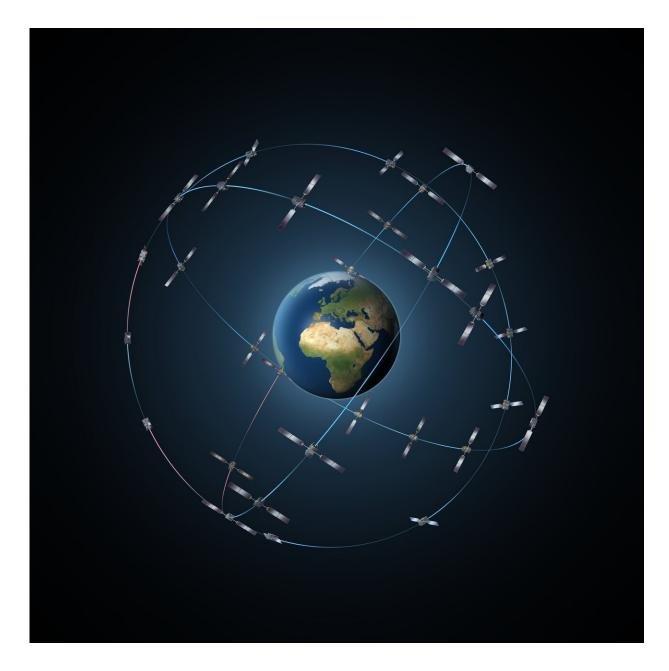
The complete Galileo constellation will consist of 24 satellites along three orbital planes, plus two spare satellites per orbit. The result will be Europe's largest-ever fleet, providing worldwide navigation coverage. Credit: ESA-P. Carril
