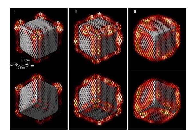
3D reconstruction of the electromagnetic field surrounding a magnesium oxide nanocube. The three modes (I, II, III) represent the nanocube's different energy absorptions. Credit: G. Habelferner, Graz univ.
