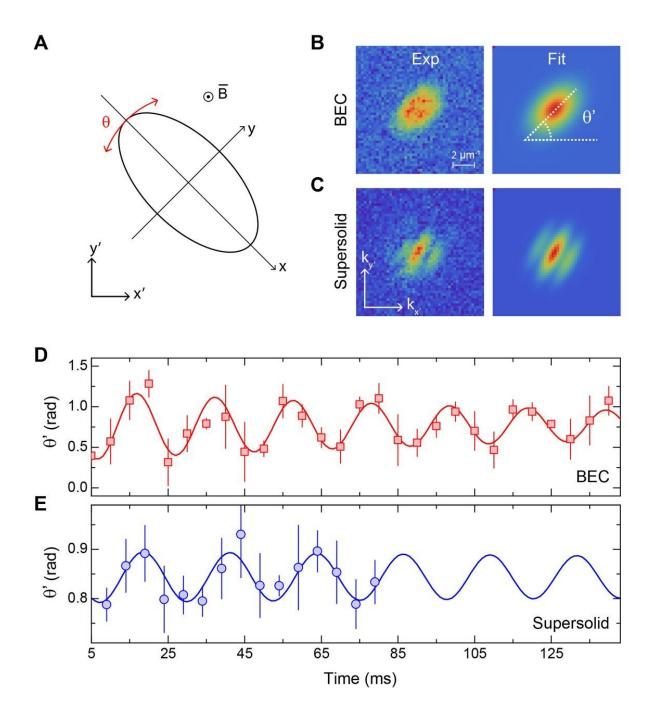
Scissors mode measurements. A) Sketch of the experimental geometry: the atomic system (ellipse) is trapped in an anisotropic potential with eigenaxes x and y. A sudden rotation of the trapping potential excites an angular oscillation  $\theta(t)$  (red arrows). B-C) Examples of the experimental distributions after free expansion and of the corresponding two-dimensional fits used for extracting the oscillation angle  $\theta$  0 after the free expansion in B) BEC regime (dd=1.14); C)
