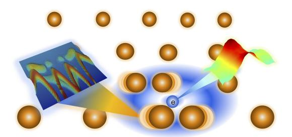
An electronic instability destabilizes the lattice, triggering charge-density wave and inducing Kohn anomaly. Credit: Aditya Prasad Roy, Department of Mechanical Engineering, IIT Bombay
