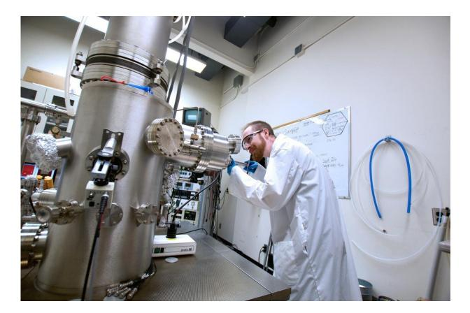
University of Toronto graduate student Matthew Timm prepares scanning tunneling microscope for an experiment controlling the outcome of a chemical reaction in by selecting the impact parameter of molecular collisions. Credit: Diana Tyszko
