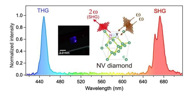
Figure 1. The nonlinear emission spectrum from diamond crystal with NV centers (NV diamond) excited with IR laser (1350 nm). Both SHG and THG are simultaneously generated at 675 nm and 450 nm, respectively. An inset photograph was taken during the nonlinear emission (SHG and THG) from the NV diamond. Credit: University of Tsukuba
