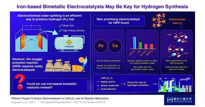
Electrochemical water splitting demands highly active, easily produced, and costeffective electrocatalysts for the oxygen evolution reaction (OER). An iron (Fe)/calcium (Ca)-basedbimetallic oxide,  $CaFe_2O_4$ , exhibits outstanding OER activity in alkaline media.  $CaFe_2O_4$  is expected to be a promising OER electrocatalyst for water splitting. Credit: Tokyo Tech
