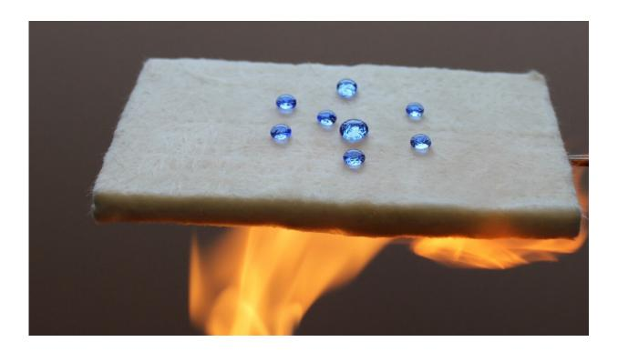
French company Keey Aerogel can produce its aerogel thermal insulation at around half the cost by extracting silica from waste concrete rather than using new silica. Credit: Keey Aerogel
