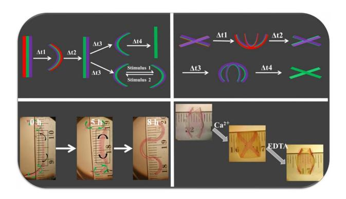
4D hydrogel-based materials can undergo multiple conformational shape changes in response to environmental cues. Credit: Aixiang Ding
