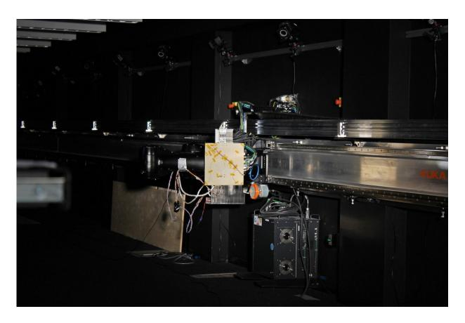
The reduced version of the LED target plate for Proba-3 vision-based sensor system testing, mounted on the robotic arm in the GRALS facility. Credit: ESA
