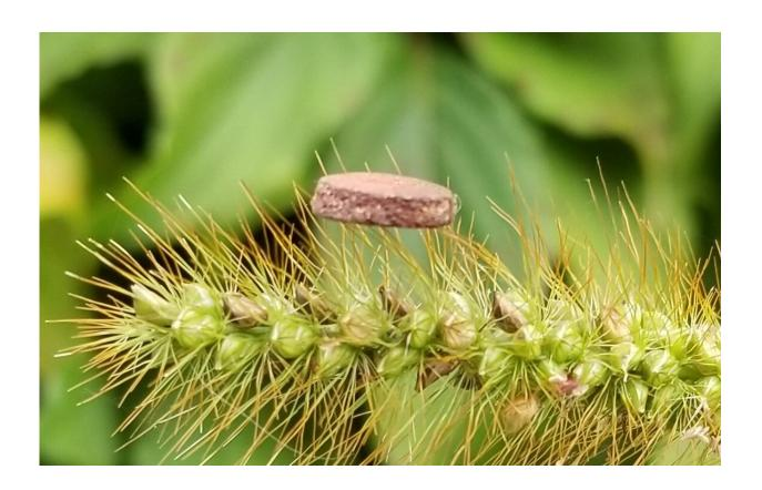
A copper-based foam filter that could someday be used in facemasks or air cleaners sits on the bristles of a plant, illustrating its light-weight nature. Credit: Adapted from *Nano Letters* 2021, DOI: 10.1021/acs.nanolett.1c00050
