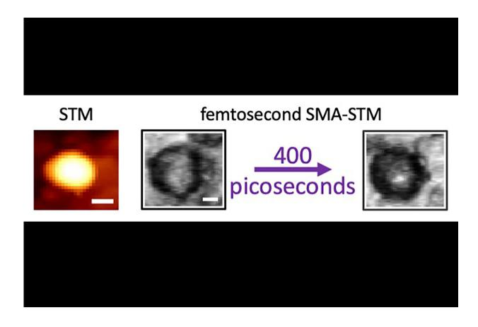
The ordinary scanning tunneling microscopy image of a carbon dot on the left shows only a featureless dot. The time-resolved single molecule absorption STM on the right reveals that laser excitation is initially spread over the whole carbon dot, but within a few picoseconds the excitation migrates to a highly localized area on the surface. The white scale bar is 5 nanometers long. Credit: Martin Gruebele
