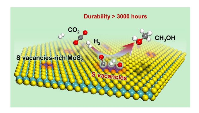
Researchers achieved for the first time low-temperature high-efficiency hydrogenation of CO2 to methanol, with a long working life over sulfur vacancy-rich few-layered MoS2, as well as remarkably higher activity and selectivity than those of the commercial Cu/ZnO/Al2O3 catalyst. Credit: DICP
