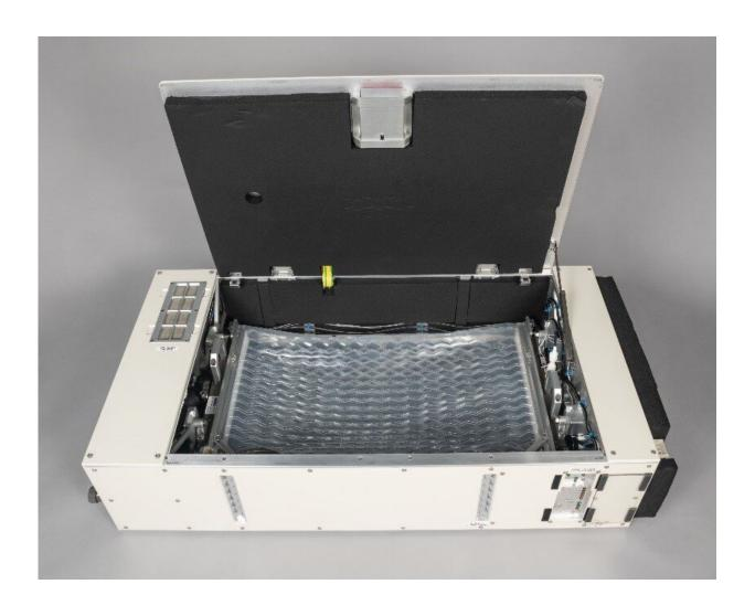
Brine Processor Assembly (BPA). The BPA's dual-membrane bladder works to recover additional water from urine brine. Credit: NASA/Robert Markowitz
