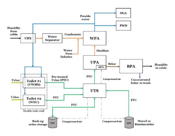
This diagram shows how the BPA fits into the water system. Credit: NASA
