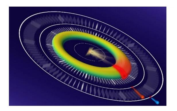
Artistic depiction of XFEL measurement with neon gas. The inherent delay between the emission of photoelectrons and Auger electrons leads to a characteristic ellipse in the analyzed data. In principle, the position of individual data points around the ellipse can be read like the hands of a clock to reveal the precise timing of decay processes. Credit: Daniel Haynes and Jörg Harms/Max Planck Institute for the Structure and Dynamics of Matter.
