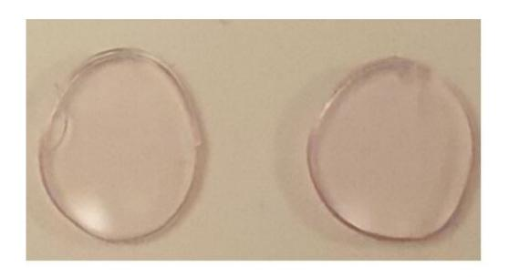
Rose-tinted contact lenses (about 10 mm in diameter) containing gold nanoparticles filter out problematic colors for people with red-green color blindness. Credit: Adapted from *ACS Nano* 2021, DOI: 10.1021/acsnano.0c09657
