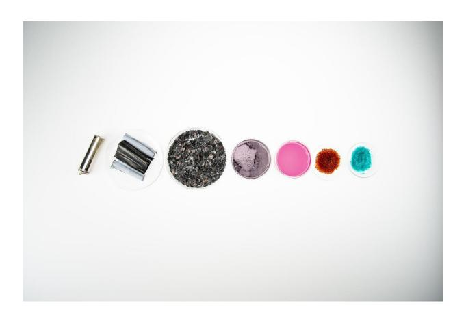
With new solution-based recycling processes, more raw materials can be recovered from batteries. In the picture, a red cobalt salt and a blue-green nickel salt have been obtained from a battery cell. Credit: Valeria Azovskaya/Aalto University
