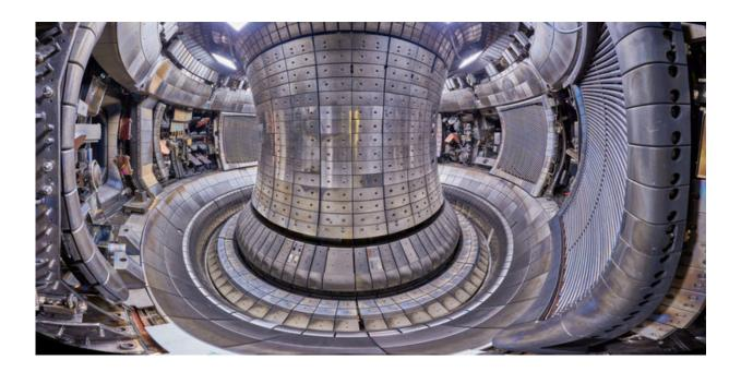
The plasma vessel from Asdex Upgrade. At the bottom you can see the divertor's baffle plates. Credit: Volker Rohde
