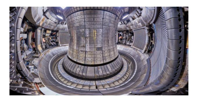
The plasma vessel from Asdex Upgrade. At the bottom you can see the divertor's baffle plates. Credit: Volker Rohde
