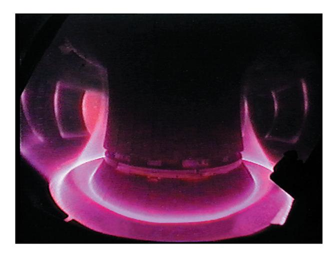
View into the plasma of Asdex Upgrade. The edge of the plasma is directed onto the robust divertor plates at the bottom of the vessel. Credit: MPI for Plasma Physics
