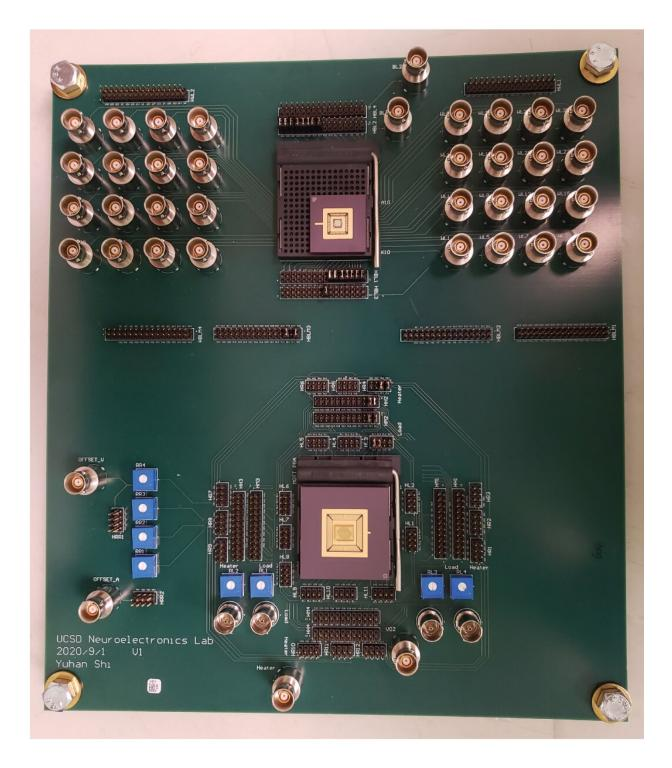
A custom printed circuit board built with an array of activation (or neuron) devices and a synaptic device array. Credit: Sangheon Oh/Nature Nanotechnology
