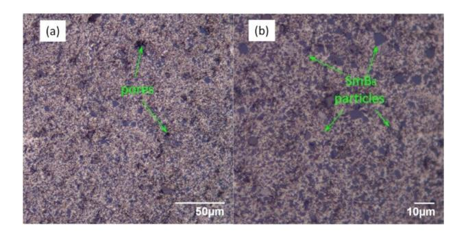
Typical optic micrographs of the composite material Credit: Serebrennikov et al. / Results in Physics, 2021
