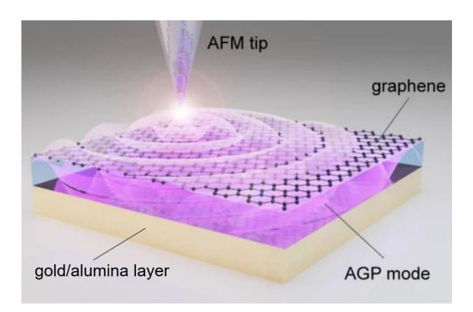
Laser-illuminated nano-tip excites the acoustic graphene plasmon in the layer between the graphene and the gold/alumina. Credit: The Korea Advanced Institute of Science and Technology (KAIST)
