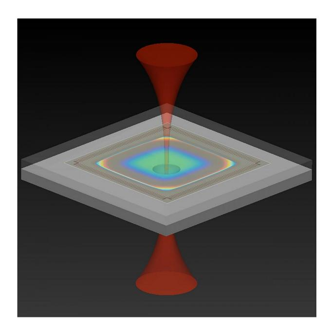
Illustration of an optomechanical accelerometer, which uses light to measure
