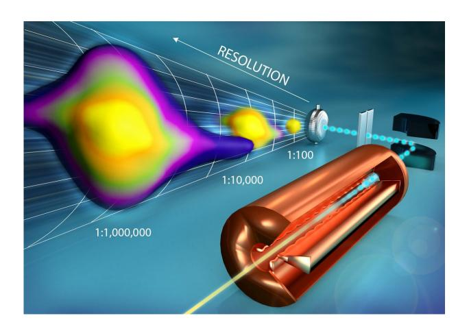
The illustration traces the path of the beam as it passes through the copper radio frequency quadrupole, the black dipole magnet, and the slitted measuring system, and onto the particle detector. The beam's structural complexity increases when measured at progressively higher resolutions. Credit: ORNL/Jill Hemman
