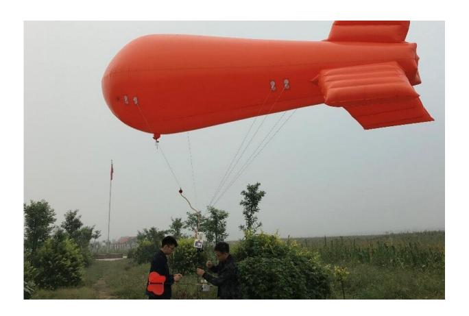
Scientists prepare to release the tethered balloon to sample the lowest layers of the atmosphere. Credit: Guiqian Tang
