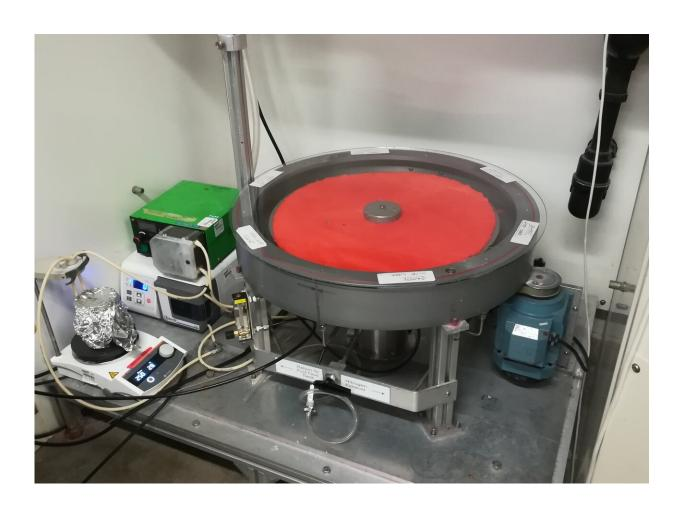
The engineers behind the Spinning Mesh Disc Reactor have won funding to continue developing their innovative catalytic reactor. Credit: University of Bath
