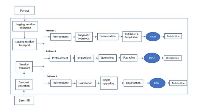
Fig. 1. System boundary used in the case study. *Energies* (2020). DOI: 10.3390/en13246701
