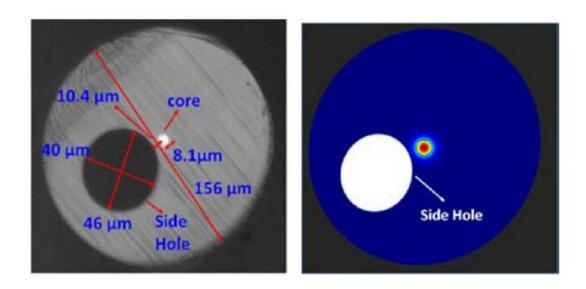
Researchers developed an extremely sensitive miniaturized optical fiber sensor that can measure small pressure changes. Adding a side hole that runs parallel to the fiber core enhanced the pressure measurement and accuracy. Credit: Xin Cheng, The Hong Kong Polytechnic University
