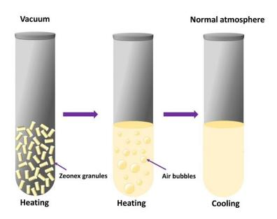
The optical fiber used to make the new sensor is made completely of the advanced polymer Zeonex. The diagram shows how the researchers made the preform that was then heated and pulled to make the fiber. Credit: Xin Cheng, The Hong Kong Polytechnic University
