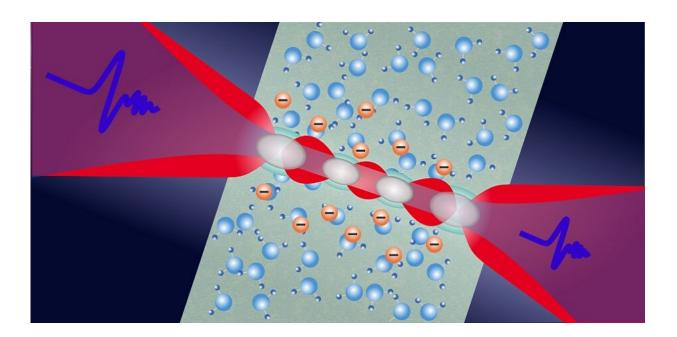
THz spectroscopy probes photoexcited plasma in water. Credit: Tan et al., doi 10.1117/1.AP.3.1.015002
