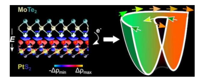
he image at left shows the crystal structure of a MoTe2lPtS2 heterobilayer with isocharge plots from a model created at Rice University. When the materials are stacked together, mirror symmetry is broken and there is a charge transfer that creates an intrinsic electric field. This field is responsible for Rashba-type spin-splitting shown by the band structure at right, where the spin is perpendicular to momentum. Credit: Sunny Gupta
