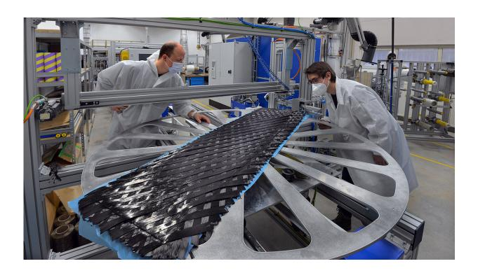
Jakob Schmidt and Marc Fleischmann, research assistants at the Department of Textile Technologies at Chemnitz University of Technology, check the quality of a splitboard's preform on the turntable of a special system. This near-net-shape preform was manufactured using the dry fiber placement process, in which the carbon fibers are placed on top of each other to save material. Credit: Chemnitz University of Technology
