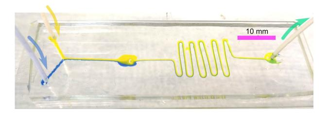
Dye-mixing inside a microfluidic chip made using 3D-printed interconnecting channel scaffolds. Credit: University of Bristol
