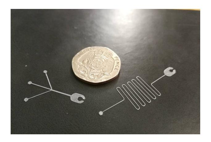
Example 100-micron wide 3D-printed microchannel scaffolds, shown next to a 20p coin - the cost to print 1000 of these channels. Credit: University of Bristol
