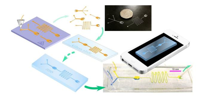
Simplified flow-diagram of the low-cost technique for fabricating microfluidic devices. Resulting channels can be applied directly to a glass surface with no additional treatment. Credit: University of Bristol
