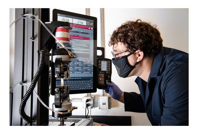
NREL researcher Nic Rorrer tests a sample of a new plastic formulation for its tensile properties. As part of Gregg Beckham's plastics research group, Rorrer is working on the redesign of nylon (aka polyamide) polymers so they can be chemically recycled with more efficient and less energy-intensive processes. Credit: Dennis Schroeder, NREL
