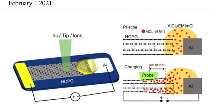
Schematic of the Al/HOPG planar model battery. Credit: @Science China Press
