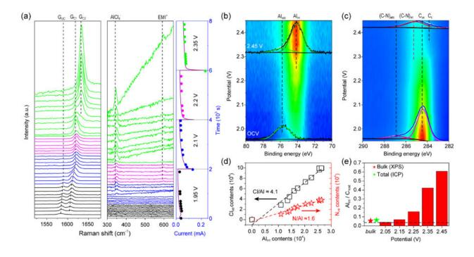
(a) Operando Raman measurements. (b) and (c) Operando XPS results of Al 2p and C 1s, respectively. (d) Dependence of intercalated Cl (Clint) and intercalated N (Nint) contents with intercalated Al (Alint) contents. (e) Atomic ratios between intercalated Al (Alint) and host-C (Chost) at different potentials. The theoretical value (dash line) and the concentration in bulk (red and green stars) are displayed for reference. Credit: @Science China Press
