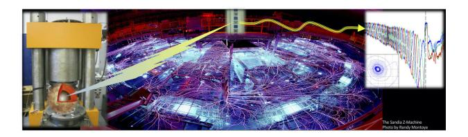
An illustration showing how a combination of static high-pressure synthesis techniques and dynamic methods enabled the researchers to probe the magnesium silicate bridgmanite, believed to be predominate in the mantles of rocky planets, under extreme conditions mimicking the interior of a super-Earth. Credit: Yingwei Fei. Sandia Z Machine photograph by Randy Montoya, Sandia National Laboratories.
