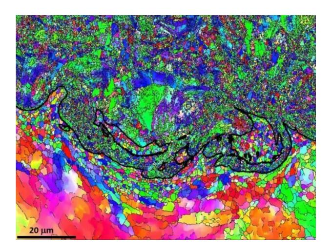
The upper part shows a cold spray copper coating, with very visible vortex-like structures twirling around an aluminium substrate in the bottom part. Credit: EBSD
