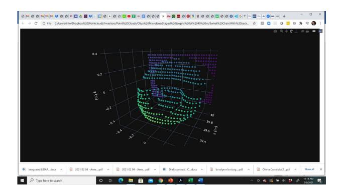
Swivel chair and screen at 40 m -- picture taken using a 32x16 pixel sensor (2mmx2.5mm sensor size). Credit: Pointcloud Inc
