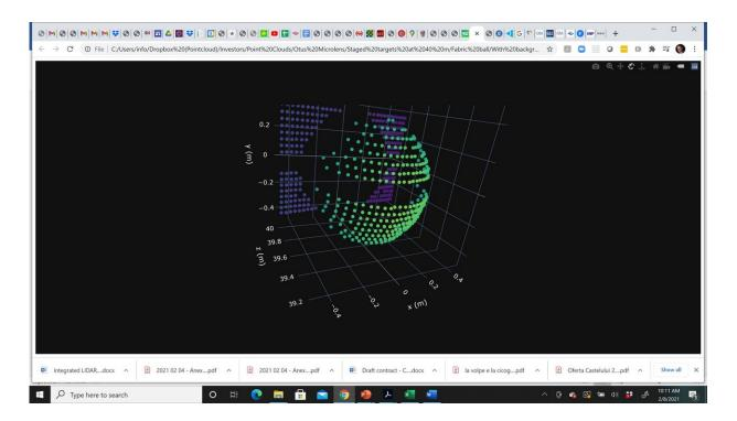
Exercise ball and screen at 40 m -- picture taken using a 32x16 pixel sensor (2mmx2.5mm sensor size). Credit: Pointcloud
