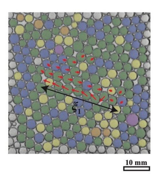
A rearrangement event in a monodisperse foam. Note how bubbles move in the same direction along the same row, or in exactly the opposite direction in
