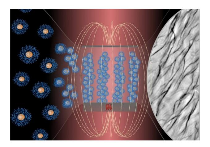
Filaments made of polymer-coated iron oxide nanoparticles are obtained by exposing the material to a magnetic field under controlled temperature. The applications are myriad and include transporting substances into cells or directing fluids. Credit: researchers' archive
