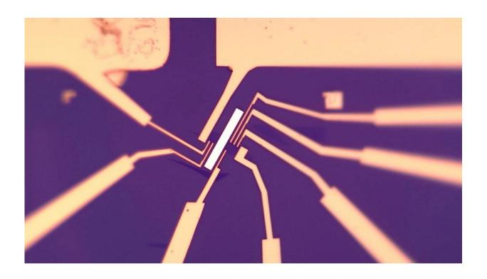
Eight electrodes around a 20-nanometer-thick magnet (white rectangle). The graphene, not show, is less than is less than 1 nanometer thick and next to the magnet. Credit: University at Buffalo.
