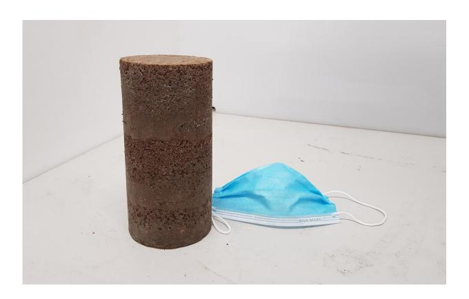
A sample of the recycled road-making material, which blends shredded single-use face masks with processed building rubble. Credit: RMIT University
