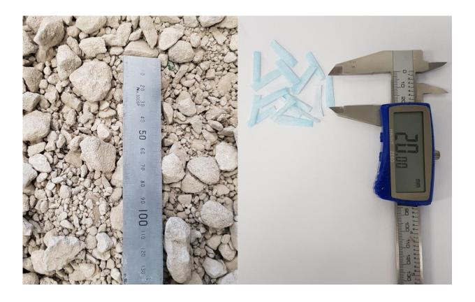
The new material blends recycled concrete aggregate (left) and small strips of shredded disposable face masks (right). Credit: RMIT University
