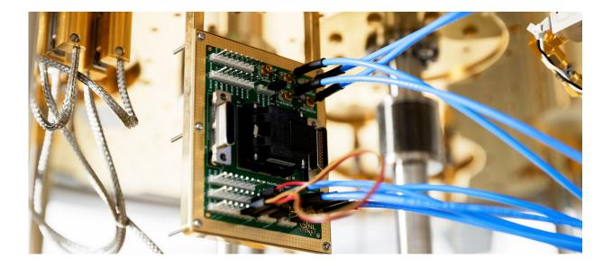
The cryogenic chip platform in situ in a dilution fridge. The device can operate at 0.1 Kelvin. Credit: University of Sydney
