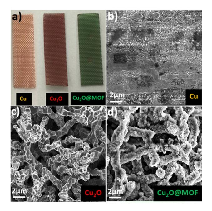
Figure a shows the images of copper wires, cuprous oxide nanowires and
