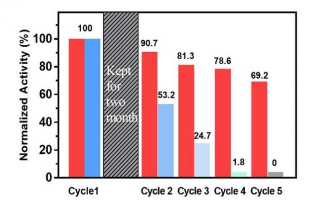
In contrast to the bare cuprous oxide sample, which lost its intrinsic activity in the fifth run, cuprous oxide with MOF shell retained 69.2% of its original efficiency for methane production after five runs. Credit: DOI: 10.1002/anie.202015735
