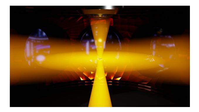
Rendering of the experimental setup (not to scale). The atoms are trapped in a single site of an attractive light sheet ('pancake') superimposed with a tightly focused optical tweezer. The system is imaged with single atom resolution through a high-resolution objective (top). Credits: Selim Jochim Group,
