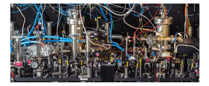
Image of the researchers' experimental setup. The main vacuum chamber with the shape of an octagon is located at the centre of the image. Here, an optical tweezer is overlapped with a light sheet trap ("pancake") in order to create a twodimensional trapping geometry for the atoms. Credits: Selim Jochim Group, University Heidelberg.
