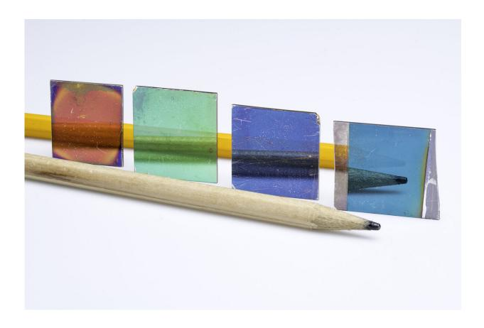
Researchers in the lab of Chunlei Guo, a professor of optics at the University of Rochester, have developed an optical coating that exhibits the same color in reflection (pictured) and transmission. Credit: University of Rochester /J. Adam Fenster
