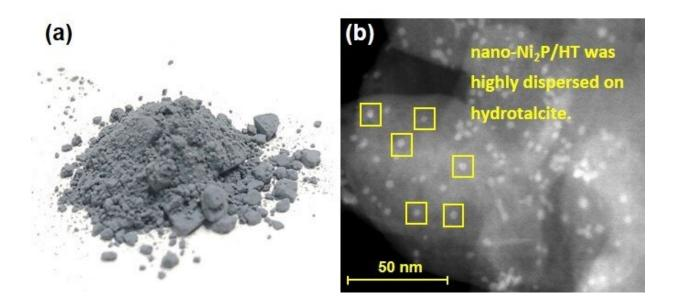
Figure 2. (a) photograph and (b) electron microscopy image of hydrotalcitesupported nickel phosphide nanoalloy (nano-Ni2P/HT). Credit: Osaka University
