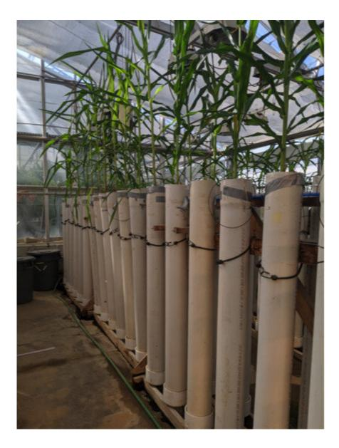
Twelve wheat genotypes and six corn genotypes were grown in a greenhouse at the University Park campus. Large growth containers, or "mesocosms," were set up with a compacted soil layer to determine which roots penetrated the hard substrate. Credit: Hannah Schneider, Penn State
